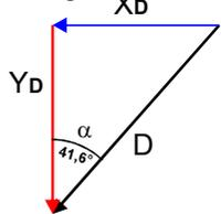
$$X_D = \sin \alpha * D = \sin 41,6^\circ * 40,14\text{kN} = 26,64\text{kN}$$
